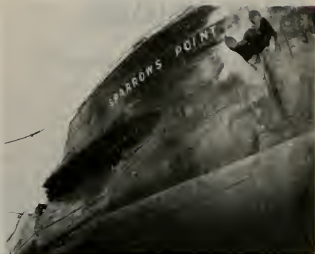
Above: Close-up view of Sparrows Point's damaged starboard bow. Below: The Escambia on drydock.
